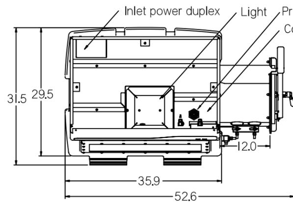
Note: Transfer chamber has a 12.0" minimum interior width
