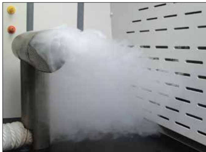
Smoke released inside the hood moves in a horizontal stream to the primary baffle slots.
