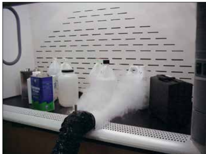
The Interior Obstructions Test simulates a typical fume hood used for chemical and equipment storage.
