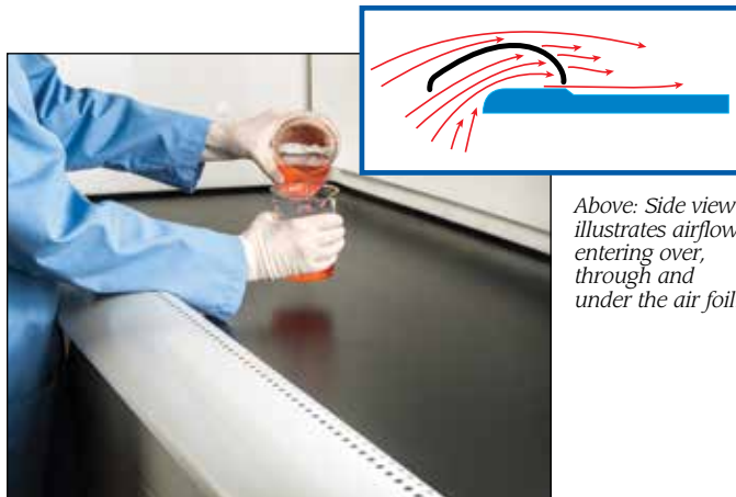
When the operator blocks the front of the air foil, air is still able to enter from under the air foil so "dead-air" zones are minimized and containment maintained.
