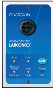
**Guardian™ Airflow Monitors.** Sense and alert the operator to low airflow conditions. From the monitor's face plate, the user can easily select and calibrate a set point between 30 and 250 fpm using user-supplied velocity meter and screwdriver. Audible/visual alarm. Includes external alarm and alarm mute functions. Flush-mount design. **Requires field calibration.**
