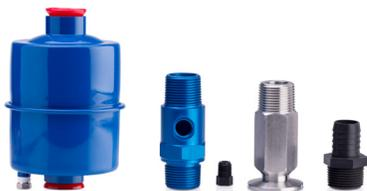
**1472200—Inlet Filter.** For rotary vane pumps 1472100, 7739400, 7739402, 1467700, 7739401 and 7739403. Prevents backstreaming and protects the pump from submicron particle damage. Includes filter assembly and one filter cartridge. Life is approximately 1000 hours at  $1.33 \times 10^{-2}$  mBar (10 microns) vacuum. Shipping weight 1.0 lb. (0.5 kg)
